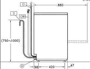
CWII Cold Water inlet 1 (cleaning) Drain ΕI Electrical inlet (power)
